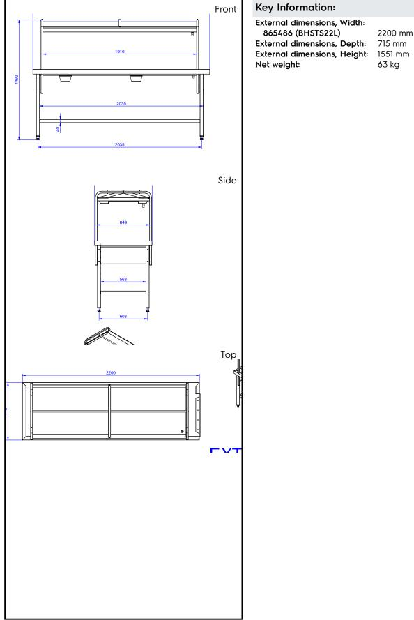
Handling System Sorting Table, Side Connection, Left to Right, 2200x715mm
